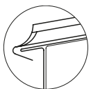
Eaves termination, standing round (favoured solution)
