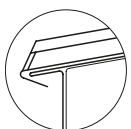
Eaves termination, standing diagonal
